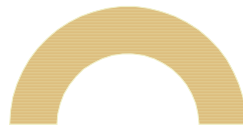
Figure 7.36: The Radial Form with its Open Space Facing South is Preferable in Palestine and Temperate Climates
