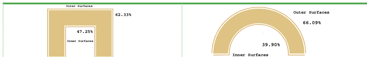
Figure 8.48: The Shaded Area Generated by the Outer and the Inner Surfaces Over the Year
